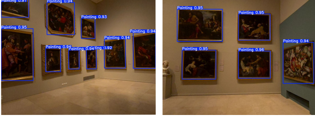
Figure 5. This figure shows some qualitative results of YOLO detection. Note that our system discard those detection that are close to borders, avoiding the projection of slice of paintings.
